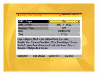
**3.Date, Time:** When select "OFF" in GMT Usage, Date and Time two items take effect, while GMT Usage turns grey. Use numeric keys to input the desired value.5. After setting, press **MENU** key or **EXIT** key to exit and save. If the value is invalid, system will inform "Invalid input! Continue to edit?". Press **OK** key at the Yes button to continue the modification, or press **OK** key at the No button to exit without saving.
